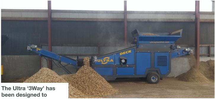
The Ultra '3Way' has been designed to offer recyclers and materials management companies a compact three grade screen that can be loaded and operated from one side, a first in a screen of this class.
